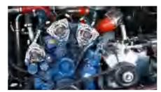
Add fireproof cover for the isolation of heat source; Layered layout of pipe lines, which is fixed and reliable; The engine is matched with a large radiator which is longitudinally placed.
